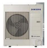
Air Source heat pumps use the refrigeration cycle to extract heat from the outdoor air and transfer it into air or into a heating fluid (normally water) for use in a building. Electrical energy is required for this process with typically, three units of heat produced for each equivalent unit of electricity. In other words, people often describe that heat pumps can operate at 300% efficiency.
